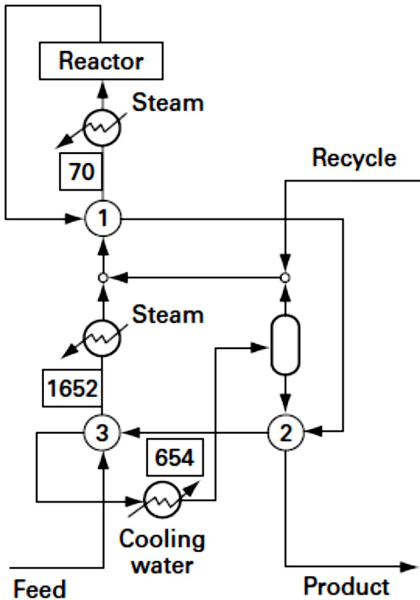
Figure 1a: A typical traditional PFD for a specialty chemicals process
