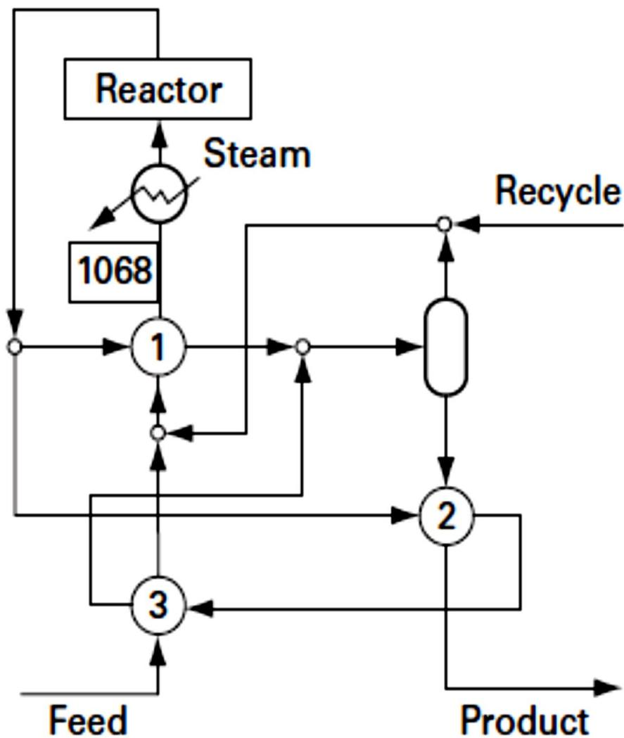
Figure 1b: A target design for a specialty chemicals process
